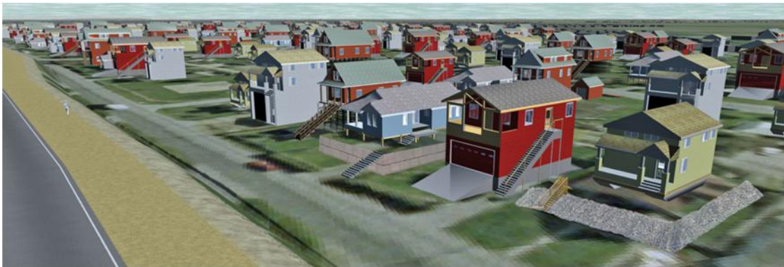
Figure 3: Examples of Raised Building Pads for Foundations 14
