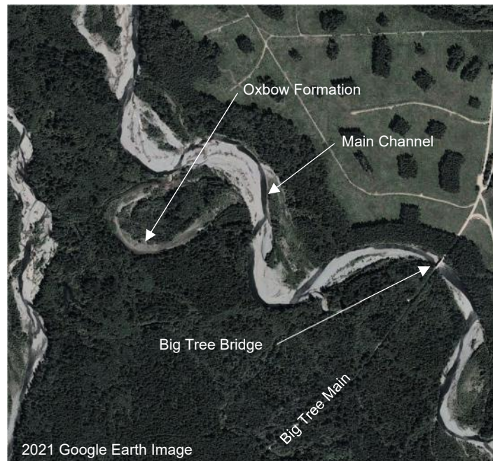
Figure 8: Oxbow Formation Downstream of Big Tree Bridge
